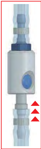
The plug is pushed toward the socket
