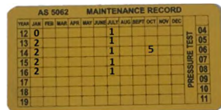
Figure 40 Service maintenance record label/tag
