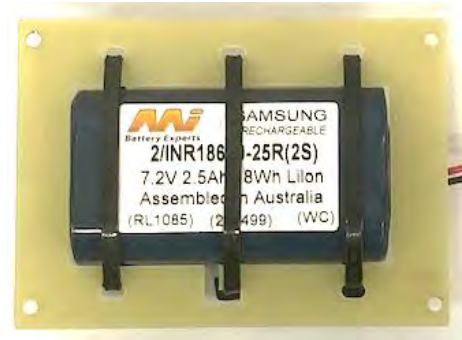
Figure 41 Back Up Battery
