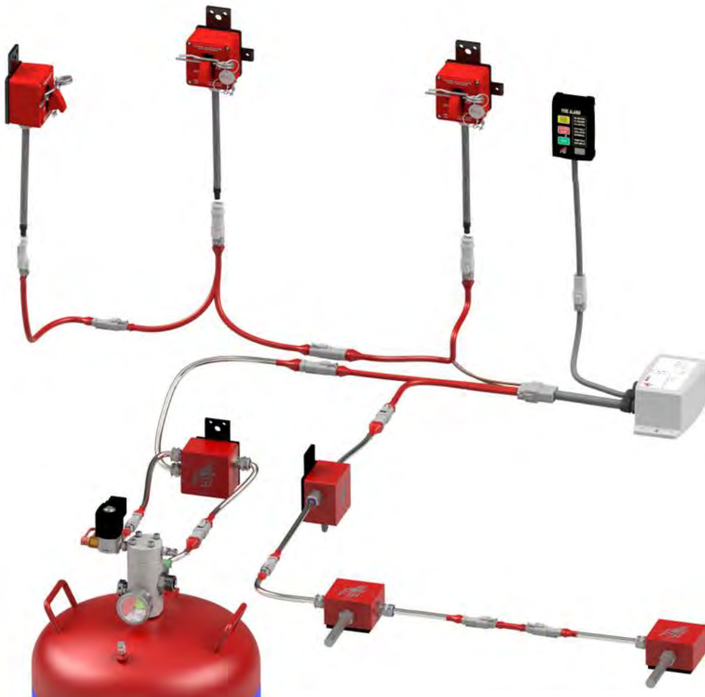
Figure 4 Electric Actuation System Layout
